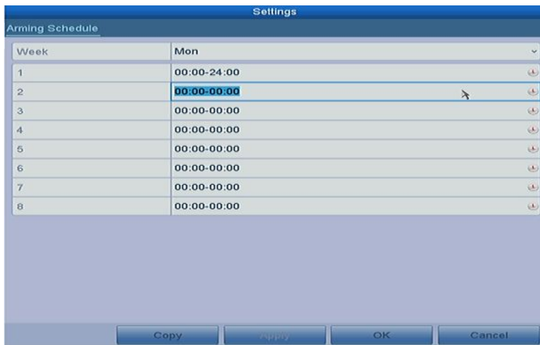
Figure 8. 16 Set Arming Schedule of Alarm Output
