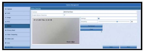
4. We can now draw our desired motion detection area on the camera preview. Use the mouse cursor to drag and draw your motion detection areas. The areas with the red grid will detect motion and will trigger your recording or email notification. You can have any amount of areas created, or use the Full screen button to make the entire view a motion detection area. The clear option will remove all areas.
