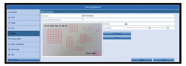
5. Once we are done drawing our motion areas, we want to make sure the system will trigger your recording or email notifications. Click on the settings icon. In the Trigger Channel section, make sure the correct channel is selected that you are working on. It should match the Camera channel at the top. In this case, it would be D1.
