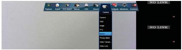
3. Select the camera, from the "Camera" dropdown at the top, that you'd like to configure and make sure the "Enable Motion Detection" box is checked.
