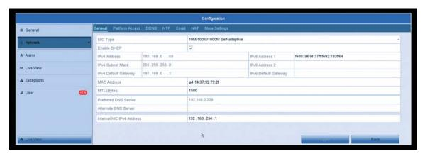
4. Then click on "DDNS" at the top. In here, we want to make sure the "Enable DDNS" box is **not** checked.
