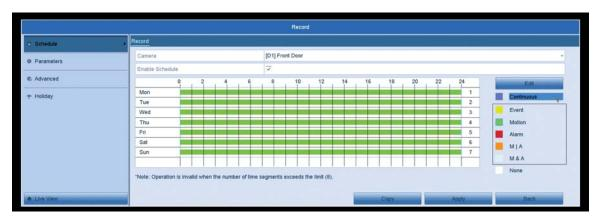
4. After selecting your desired recording type, draw a box on the sections you'd like to change. The section should change colors to the desired recording type.
