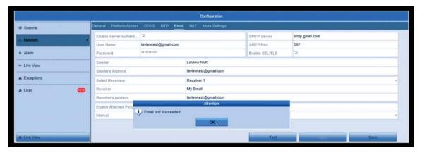
11. The NVR will now send Email Notifications out from each channel that has Motion Detection Enabled and the "Linkage Action" is setup for Email Notifications.
