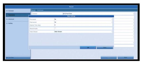
**Pre-Record:** If using "Motion Detection" recording, this will tell the system to record seconds before the motion was picked up as well as all the motion detection. System defaulted at 5 seconds and can go up to 30 seconds.
